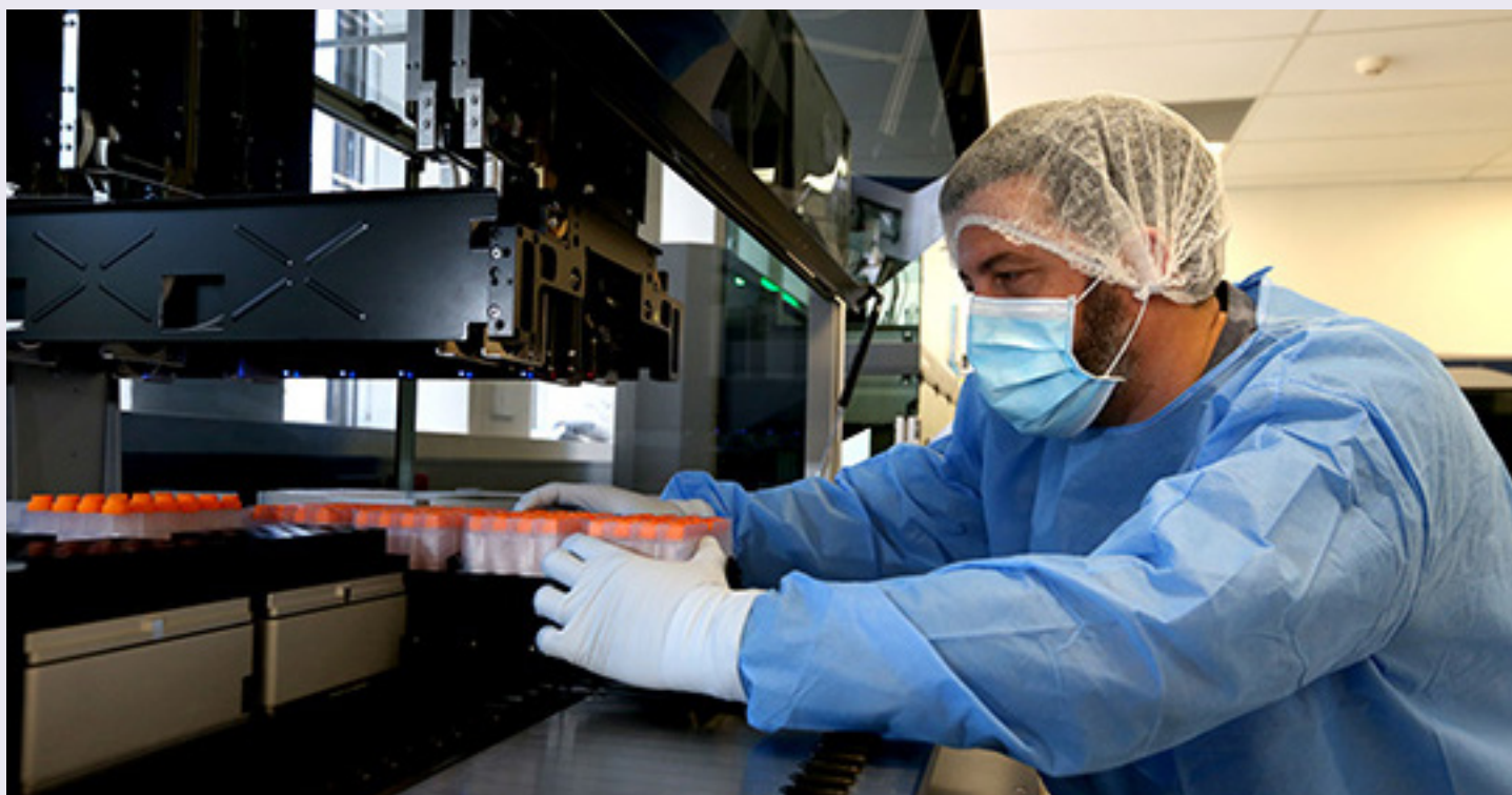
▲ DNA Scientist Allan Murray operating a robotic liquid handling platform
