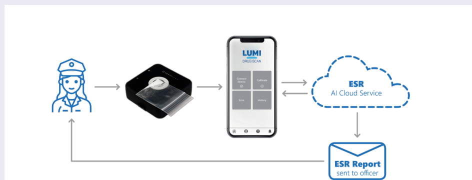
▲ The Lumi workflow: The mobile app connects the device to the cloud-hosted machine learning models, allowing the spectra from a sample to be analysed and a result provided to the officer in real-time
