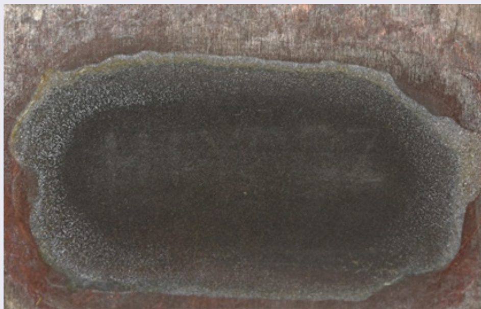
▲ Chemically Restored Serial Number HIY932
