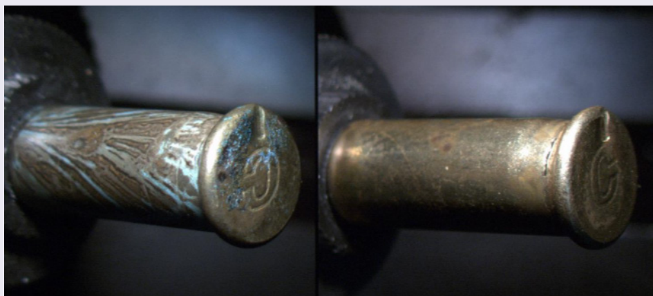
▲ Fired 22 Long Rifle calibre cartridge cases exposed to PrepFiler (Left) & QIAGEN ATL (Right) extraction buffers.
