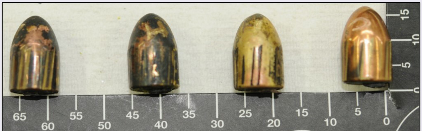
▲ 9mm Parabellum calibre copper jacketed bullets displaying corrosion after exposure to a decomposing pig analogue for approximately 2 weeks.
